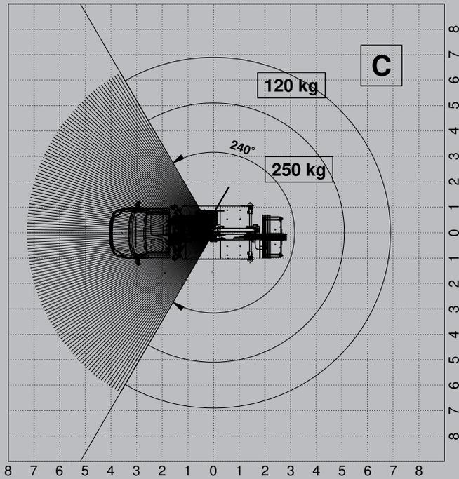
**CROSSBEAMS ONE SIDE FULLY OPENED ONE SIDE CLOSED**
