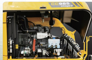
EU Stage V Compliant Engine
