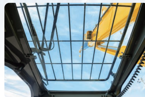
Wide View Roof Window
